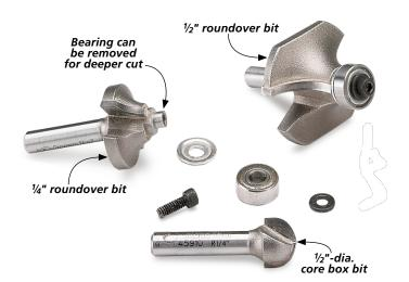
Over the years I've accumulated a lot of different router bits. The "workhorse" bits that have standard profiles get used over and over, while the more exotic "big money" bits usually just gather dust. This led me to the realization that you don't need a drawer full of expensive bits to rout complex profiles.
