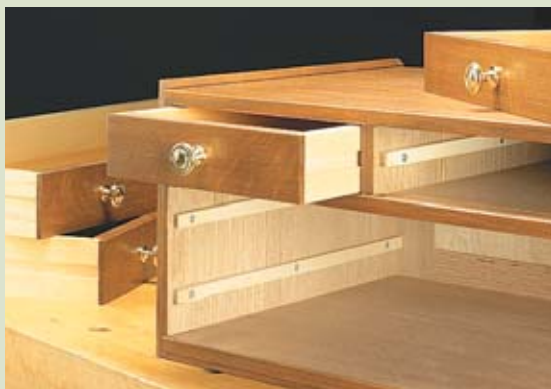
Drawer Guides. The drawers in the tool chest slide on wood runners mounted in the case. The runners fit in grooves cut on the drawer sides. A little wax will make them slide even smoother.
