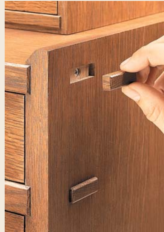
▲ The false tenons hide the screws in the cabinet sides and also add a nice detail.
