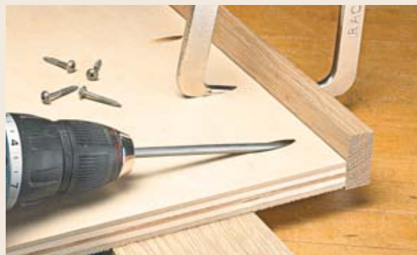
▲ Pocket holes are a great way to secure edging to a shelf. A right-angle clamp holds the edging to the shelf while the screws are driven in place.
