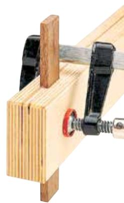
**▲ Glue Up Tip.** A waxed "key" ensures proper alignment when gluing up the fence pieces.
