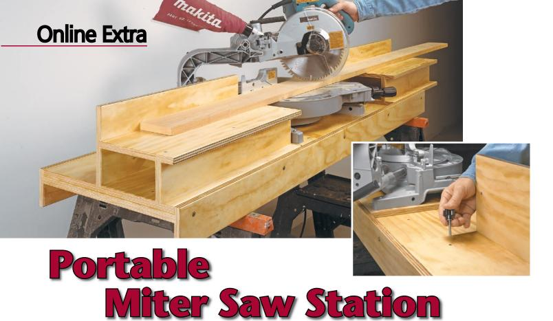
A sliding compound miter saw is a valuable addition to any shop. But like any tool, it can always be upgraded to give you better results and more convenient use. Building the workstation you see in the photo above will do just that. The workstation provides a sturdy base
