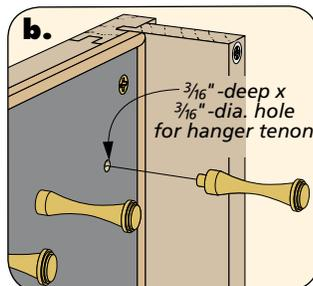
The recesses behind the doors of the tool chest featured in Woodsmith No. 168 offer versatile hanging storage space. To make the best use of this space, you might want to add one or two of the door panels shown above. These thin panels give you more flexibility by allowing you to easily attach holders for tools (or jewelry) at any spot on the back of the door.
