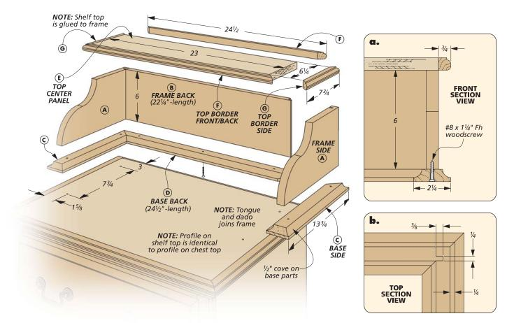
back, being careful to center it on the frame, both end to end and across its width (detail 'a'). Finish up with the two side pieces.
