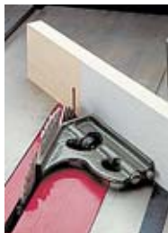
▲ Use the head of a combination square to set the miter gauge to 45°.
